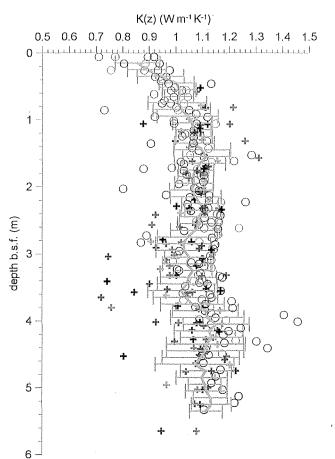
**Figure 3.** Thermal conductivity (k) measurements on cores GC-03, PC-04, PC-06, and GC-09 (open circles) and in situ (crosses) from the ridge crest area. Average interval k every 10 cm and the corresponding standard deviation were computed using a 30 cm moving window.
