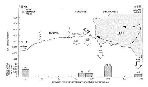
**Figure 13.** Cartoon summarizing the main results of this study, including the advance of the EMT onto the Mediterranean Ridge, the related thermal disturbance induced in the sediment, and the undisturbed thermal gradient at several locations along the corridor. Ranges of undisturbed G values reflect results from sudden and gradual warming models (see Table 2).
